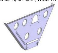
UT-03-1103-0-078 LANDING GEAR, BRACKET, WING-TYPE, CBSD
